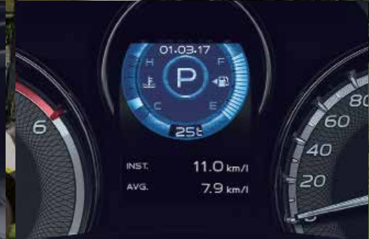
Multi Information Display shows the instantaneous and average fuel consumption
