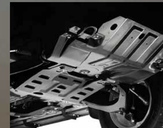
Underbody protection, front steel plate skid/shield
