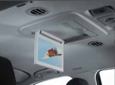
The fold-down 10.2" monitor provides a clear image display, which can be easily viewed by both the second and third row occupants.
