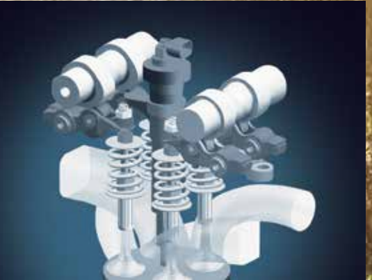
Rocker arms with large roller bearings lower friction for maximum fuel economy
