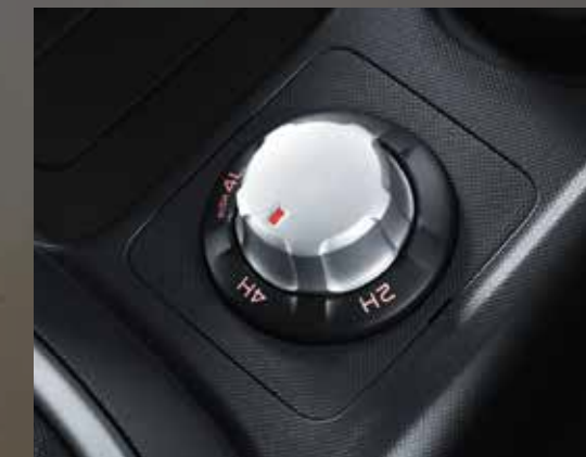
4WD select dial allows for simple shift from 2WD high, 4WD high and 4WD low
